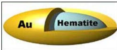
Nanorice is made of non-conducting iron oxide called hematite that's covered with gold. The core size and shell thickness vary slightly but the particles are about 20 times smaller than a red blood cell.
