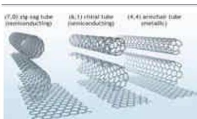
Nanotubes have different properties depending on slight differences in the way that carbon atoms are arranged.
