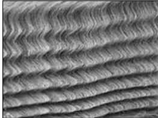
Buckled carbon nanotubes under compression. Credit: Cao/RPI
